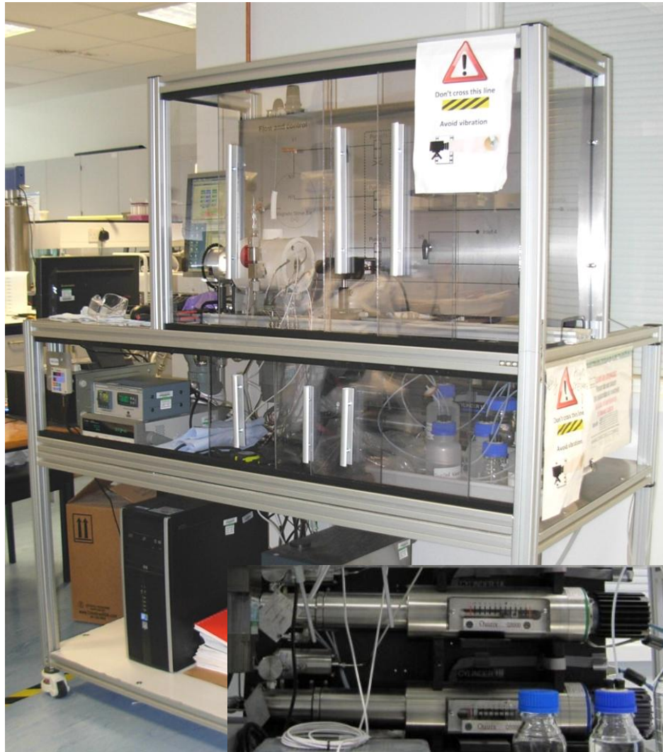
Figure 16. Experiment set-up of interfacial tension and contact angle measurement. Insert: fluid injection pumps
