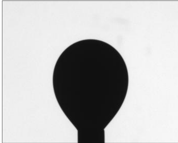
Figure 60. Crude oil sample 2 droplet in NaCl solution m = 0.07 \text{ mol}\cdot\text{kg}^{-1} , at T = 323 \text{ K} , ambient pressure
