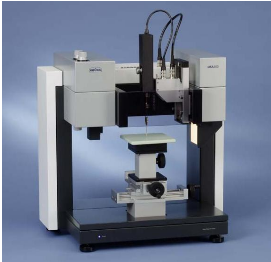
Figure 57. Instrument for interfacial tension and contact angle measurement [192]
