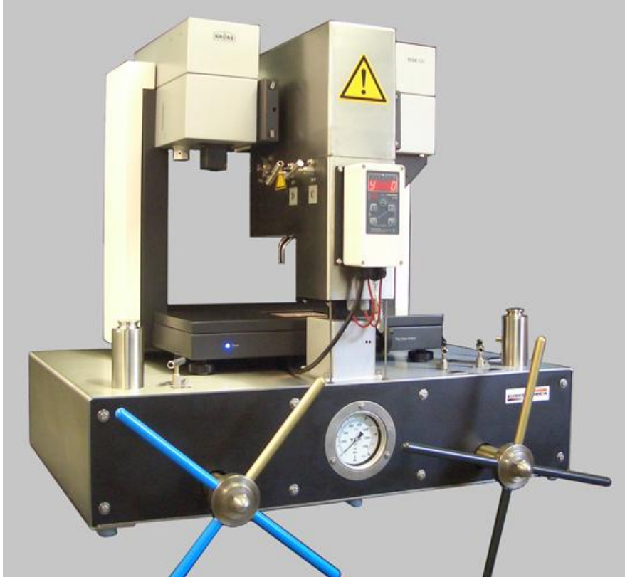
Figure 58. Instrument for HPHT interfacial tension and contact angle measurement [192]
