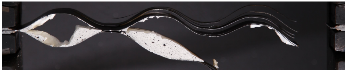
(f) After failure (note the permanent deformation in the central foam cell).
