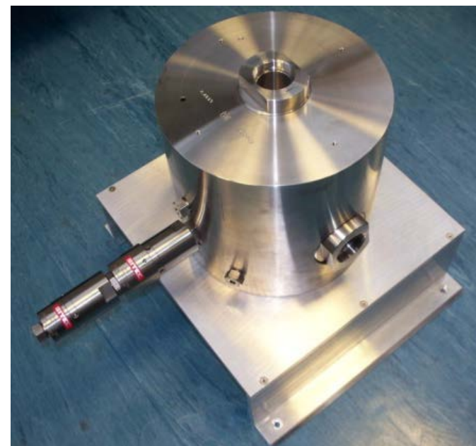
Fig. 1. Left: schematic diagram of the apparatus. Right: photograph of the high-pressure vessel showing the sapphire windows and swivel joint.
