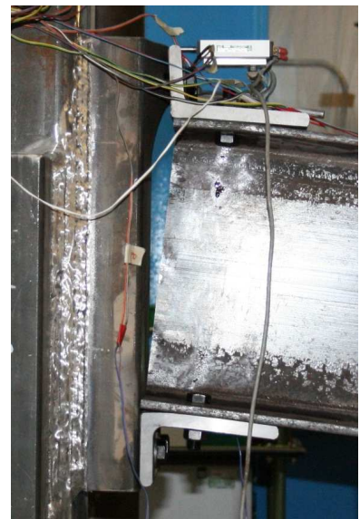
(c) Deformation at the end of test in Specimen T6.3-A15-d40-M
