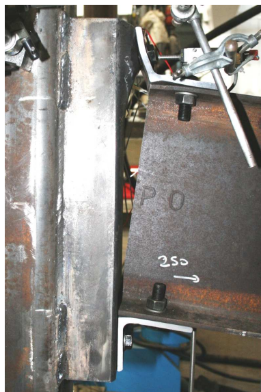
(b) Deformation at the end of test in Specimen T6.3-A8-d40-M
