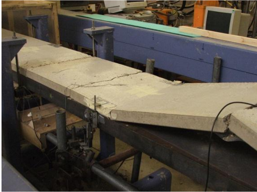
Figure 8: Strut at end of test
