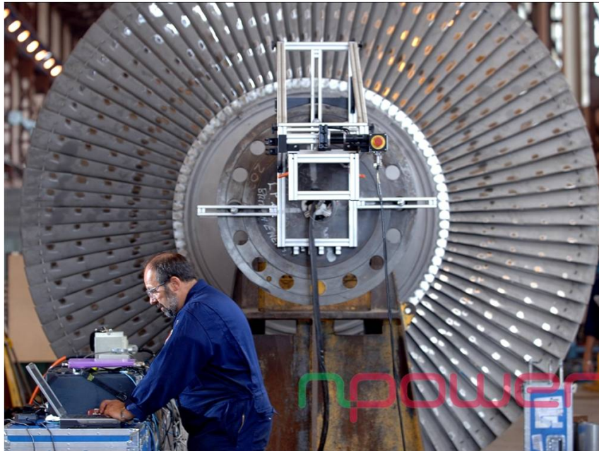
Figure 2.6: Rotor bore inspection. Some power generation rotors have a hollow bore. NDT technicians inspect the rotor by sliding and rotating an array of ultrasound and eddy current transducers through the bore. This photograph shows the frame of the probe manipulator mounted on the end face of the turbine rotor during such an inspection. (Image from [19].)
