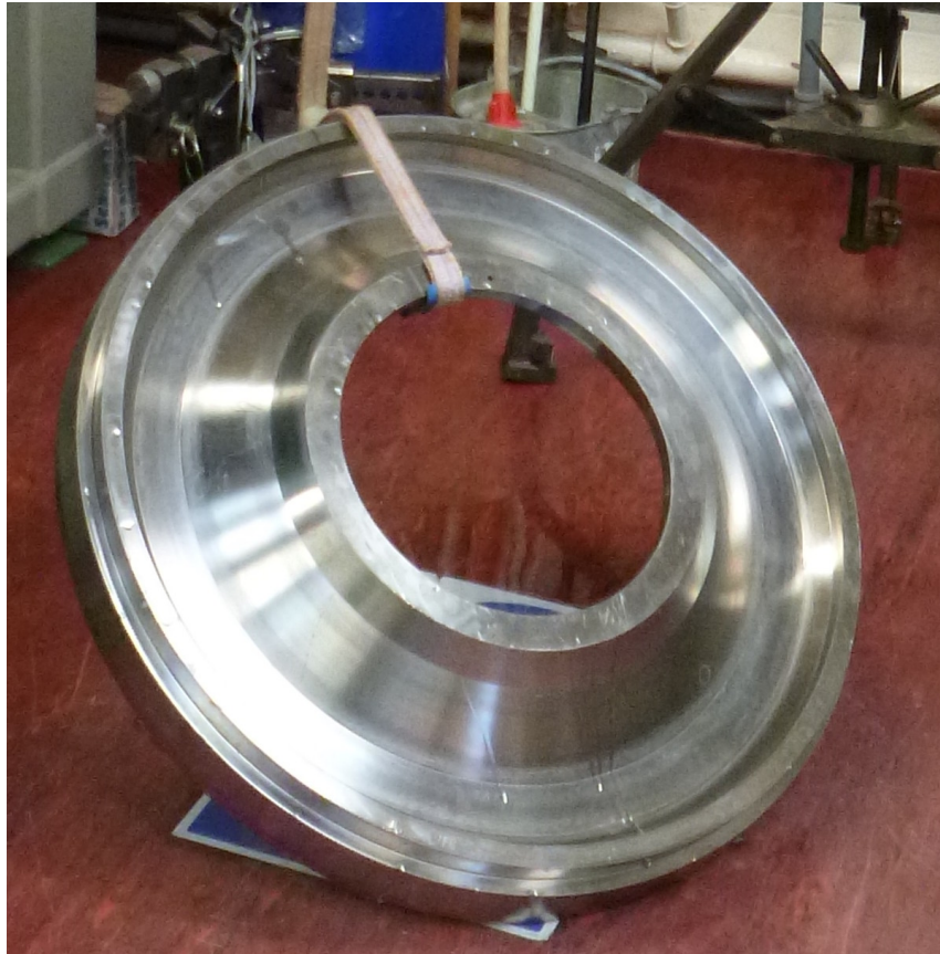
Figure 2.1: Titanium aircraft engine turbine disc. This disc is one of 3 forgings machined to the inspection shape of a Trent 890B compressor disc from a contaminated billet. The material contamination produced five known seeded defects inside the disc. Rolls-Royce uses this disc, labeled by its test piece serial number 5, to evaluate their inspection procedures and equipment. Photo: N. Brierley
