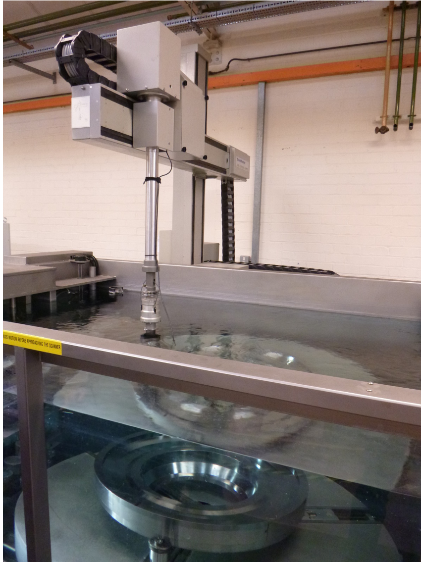
Figure 2.2: Seeded Defect Disc in the water immersion tank, ready for inspection. The disc rests on a rotating platform at the bottom of the tank. A computer-controlled, two-axis scanning frame moves the ultrasound probe radially and vertically to follow the cross-sectional profile of the disc. Photo: N. Brierley
