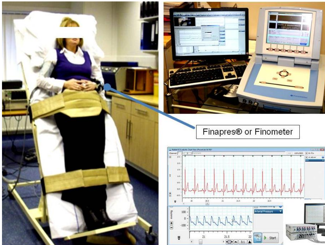
Figure 3.1. Head-up tilt table and a participant performing a 10-minute HUT (left) and examples of a beat-to-beat blood pressure recording (Finometer) and a computer with the data acquisition software (Right).
