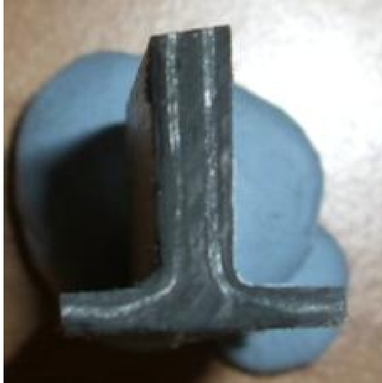
Figure 3.24.: A cross section through a long stiffener after testing appears to show a filler region with no voids or defects at the junction with the stiffener.
