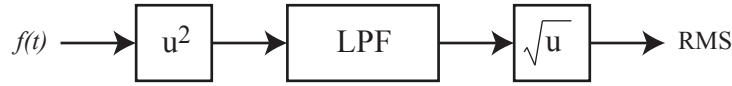
Figure 4.1: Implementation of Equation (4.8) for the RMS block used in the inverter controllers.
