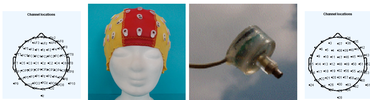
Fig 1.3 An example of a 64-electrode cap with active scalp electrodes and facial external electrodes, from the company Biosemi. From http://www.biosemi.com .
