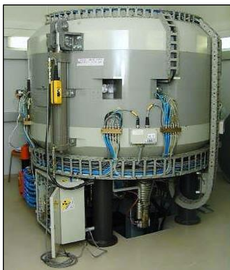
Figure 9. Example of a PET cyclotron used to produce ^{18}\text{F}
