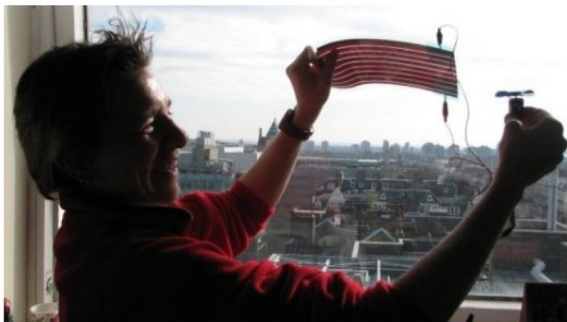
Figure 1.1. A flexible OPV device fabricated using roll-to-roll printing powers a small motor. Photo reproduced courtesy of Satchetan Tuladhar.
