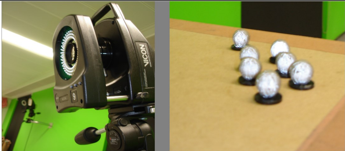
Figure 5-1 An optical motion tracking system consisting of 9 high speed cameras at an acquisition rate of 150Hz was used together with spherical reflective markers of 14 mm in diameter.
