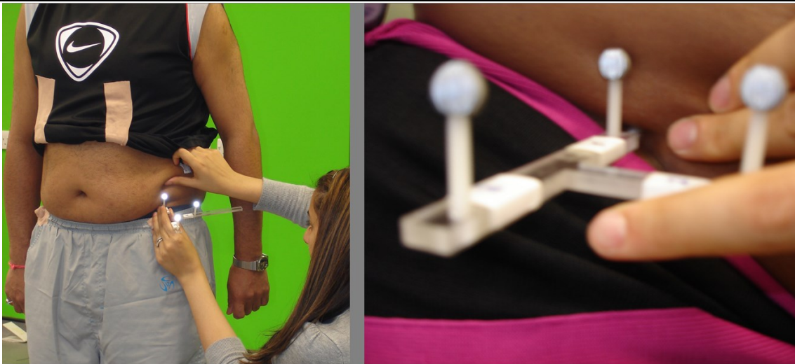
Figure 5-18 Calibrating the anatomical landmarks using the pointer enables the investigator to access the bony landmarks by pressing the tip of the pointer against the landmarks while holding the soft tissue around the abdomen
