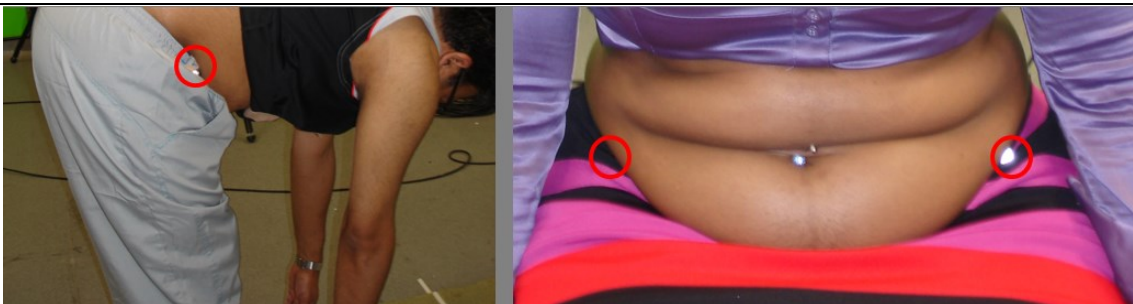
Figure 5-19 Illustration of marker occlusion during the Toe and STS activities. The red circles represent the position of ASIS markers. While the subject is seated the markers around the ASIS move relative to the underlying bone because of the soft tissue around the abdomen
