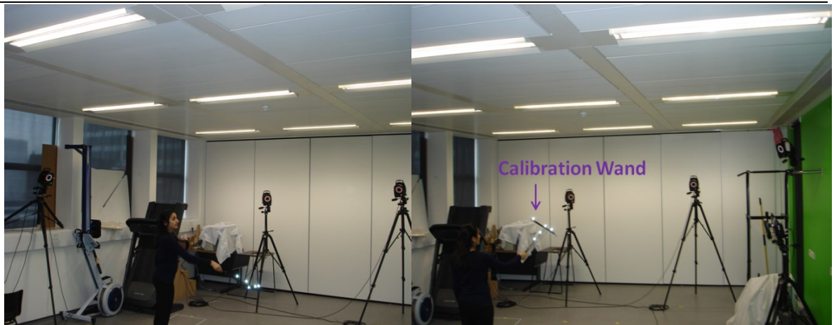
Figure 4-2 The capturing volume and the orientation and position of the cameras were calibrated by waving the calibration Wand before the experiment.
