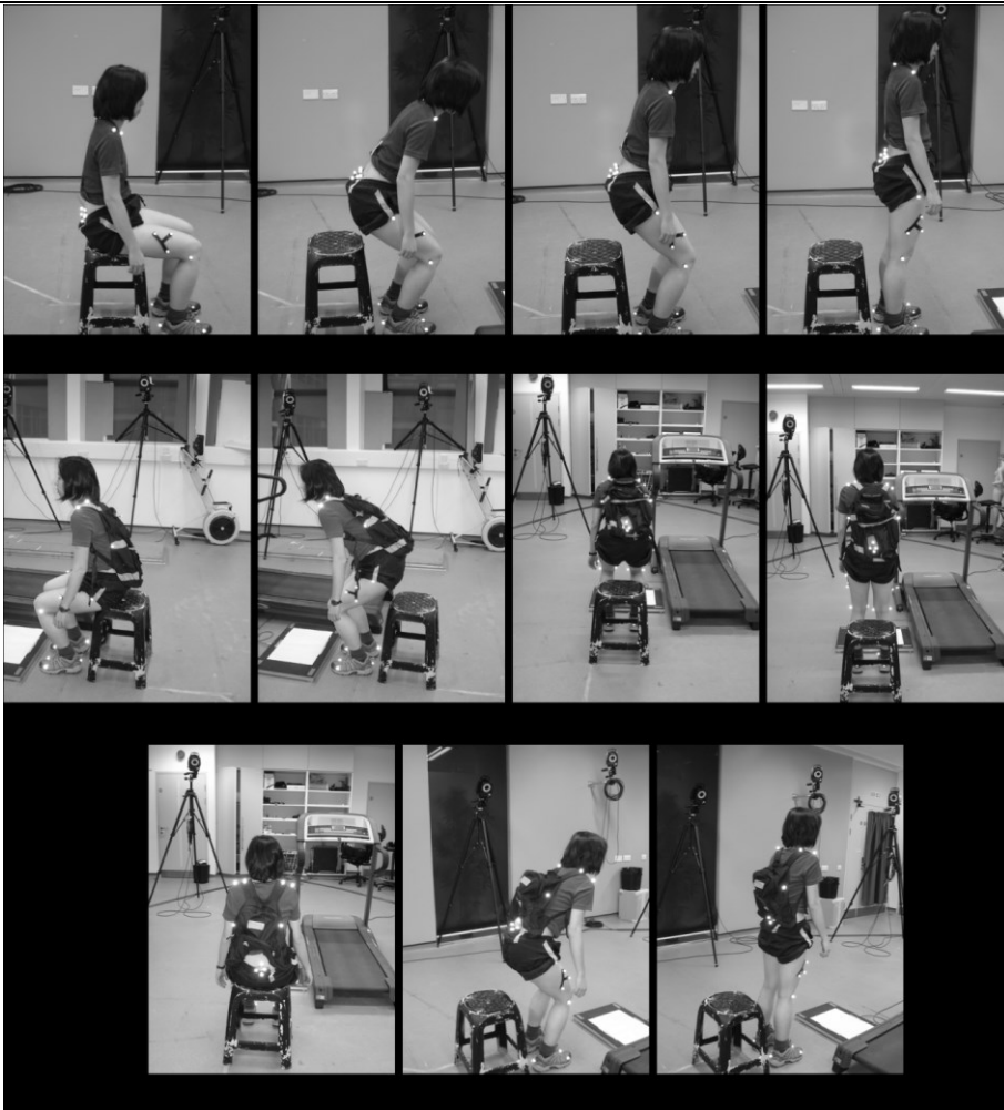
Figure 7-10 Sit-to-stand and Stand-to-sit while carrying no backpack, ERGO backpack and COMF backpack
