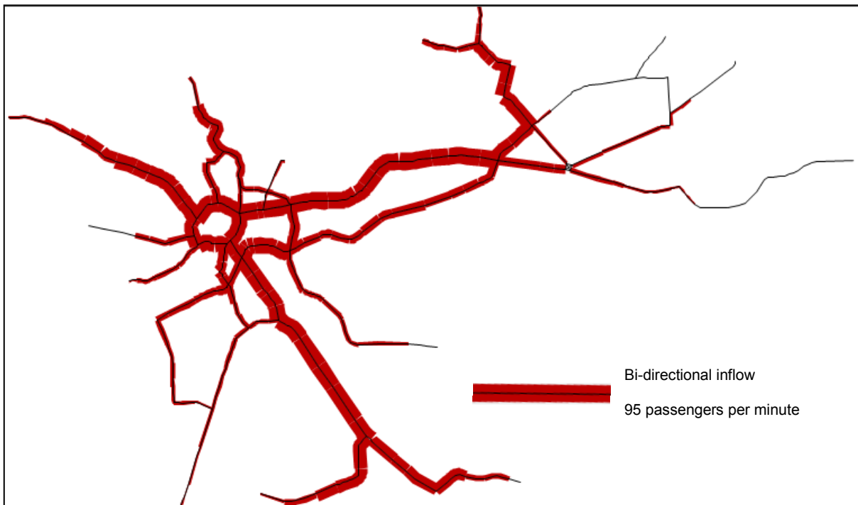
Figure 5-25 Flow pattern across the network during the 60 th time interval
