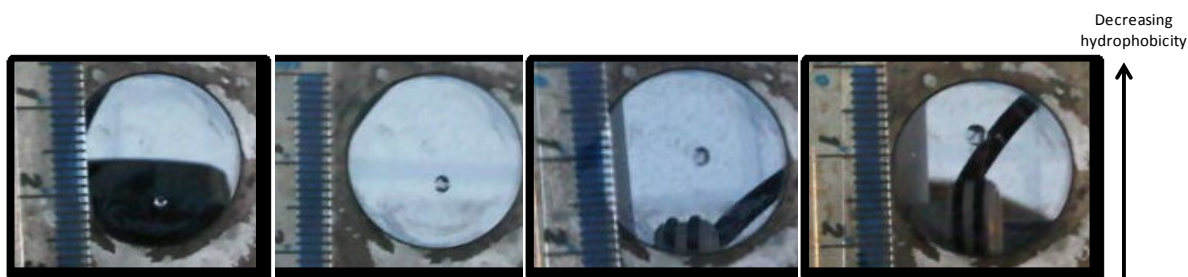
Figure 63 - Images of water droplet on the Si ATR surface with OTS gradient used to calculate contact angles.
