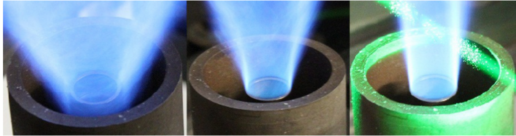
Figure 6.6: A photograph of the flame (angled view) as a function of swirl number. From left to right S=1.07 , 0.58 and 0.3 ; overall equivalence ratio is 0.9 . A position of laser sheet is also shown at y/D_f = 1 .
