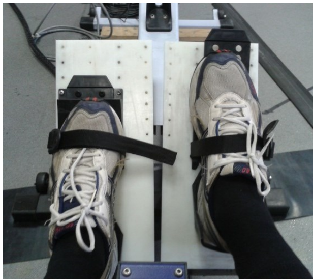
Figure 8.3: Feet constrained to the foot-stretchers at two different positions, showing the bilateral differences in placement of each strap relative to the foot.
