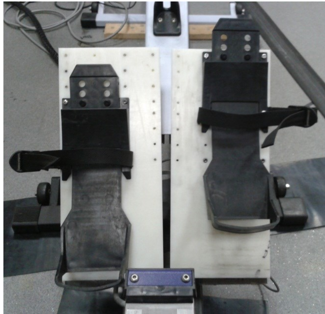
Figure 8.1: Foot-stretchers are fixed to the adjustable footplates to demonstrate two different heights. The left foot-stretcher depicts the lowest height (Position 1) and the right foot-stretcher depicts the highest height (Position 4).
