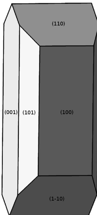
Figure 5.9: Wulff plot showing the equilibrium crystal morphology based on the relaxed surface formation energies.
