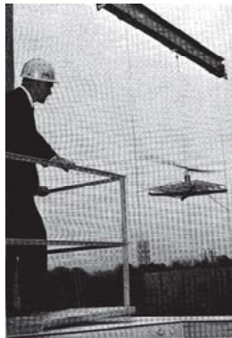
Figure 2.1: Electric rotor powered by a 400 W, 3 GHz transmitter at a distance of 20 m. [1].
