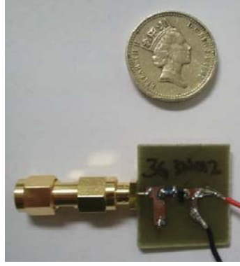
Figure 4.18: Half-wave 3G version 1 rectifier prototype on FR4 substrate [20].
