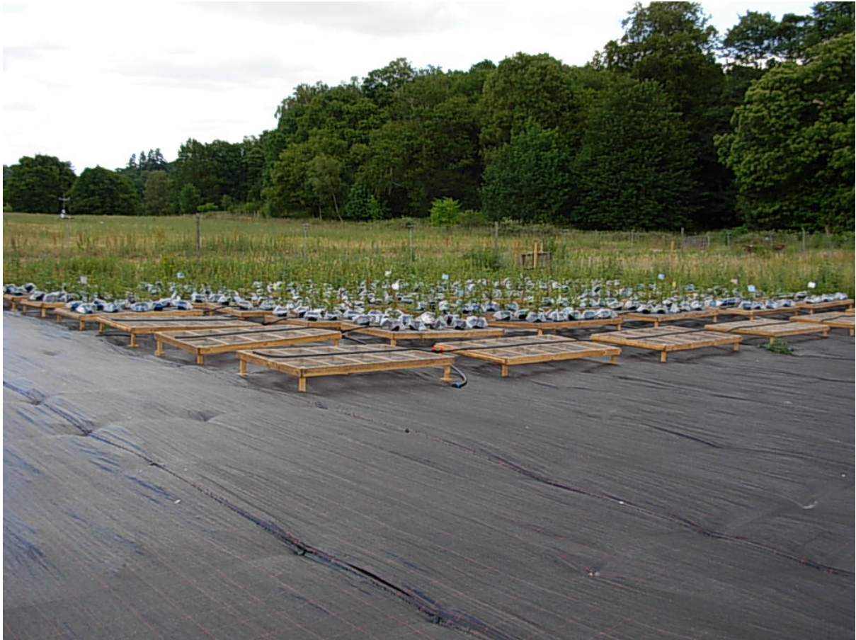
Figure 3.1: Field experiment set-up, showing 250 Sitka spruce on raised platforms in a 5 x 5 Latin square.
