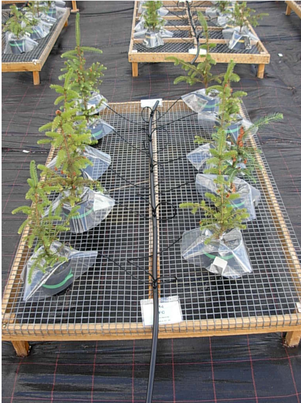
Figure 3.2: Pallet set-up in the field experiment. Ten Sitka spruce were randomly assigned to each pallet. Each pallet was assigned a drought treatment and was individually irrigated.
