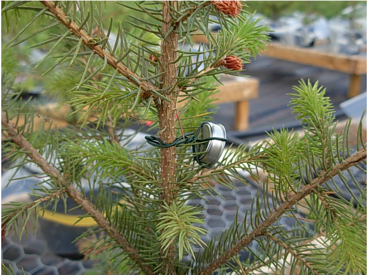
Figure A.1: A DS1921 ThermoChron iButton temperature sensor used to record temperature on the trees in the field experiment. These were attached to one randomly selected plant per pallet, and were set to take a temperature reading once per hour.
