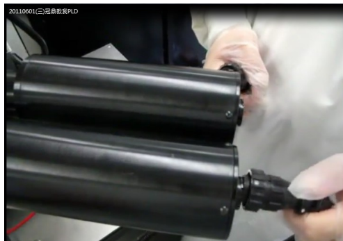
Re-connect the X and Y cables and also make sure they are at right positions
