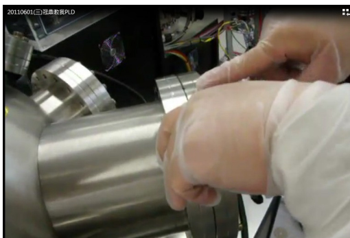
Ensure that the scribed arrow on the stainless steel rim is on top and at right position.
