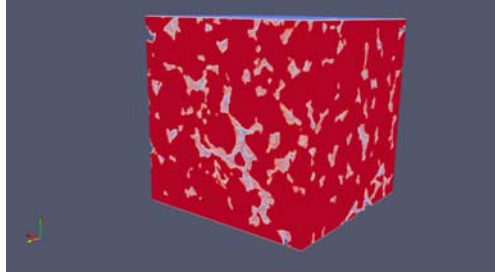
Figure 6.30.: A 3D image of Clashach sandstone with a resolution of 8.96 microns/pixel. The red represents grains while the light grey represents the pore space.
