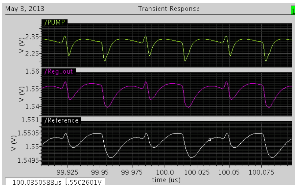
Figure 6.25: PMU steady-state behaviour showing voltage ripples. Voltage output traces at the output of the charge pump (green), the system output (regulated voltage node - pink trace) and the voltage reference output node (white).
