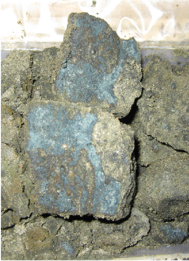
Figure 12. Green rust (bluish surface colour) in fresh core samples.
