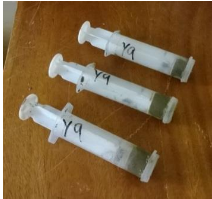
Figure 2.1 Twenty ml cut-off syringe corers with caps. Each syringe contains 3.14 \text{ cm}^3 of sediment sample ready for analysis.
