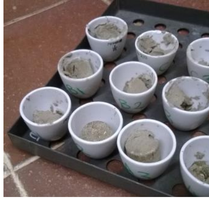
Figure 2.2 Crucibles containing syringe corers after oven drying at 105 °C for 24 hours.
