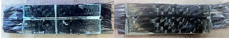
Figure 5.5. An underside view of a damaged (left) and a healed (right) vessel specimen.
