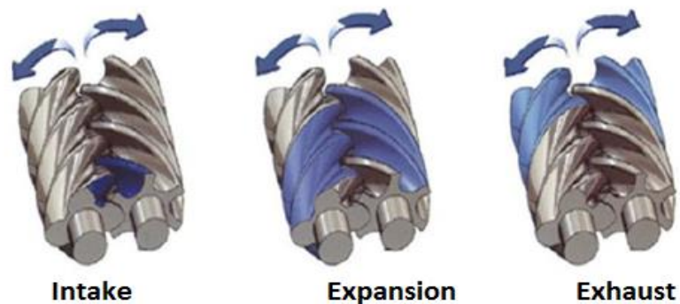
Figure 2.26 Screw expander working phases (Zhang 2014)
