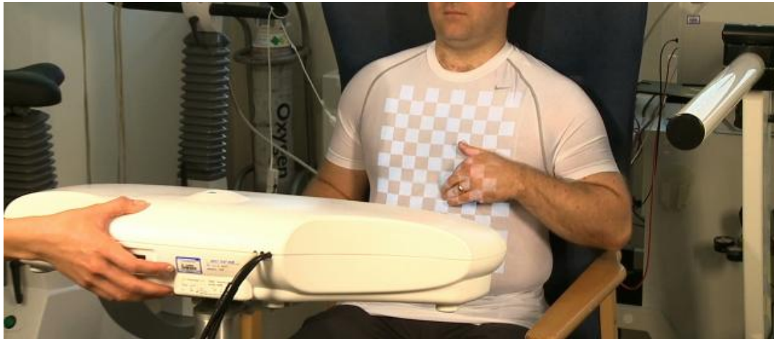
Figure 22: Example of a structured light system and pattern. Adopted from (Mair, 2012).
