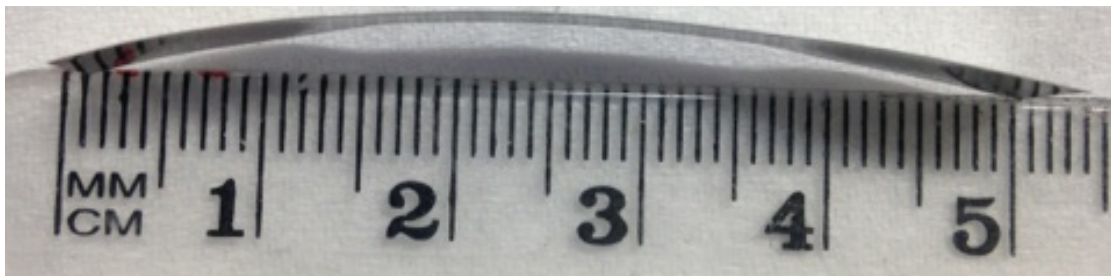
Fig 4.5.3. Photograph of film on PEEK substrate showing developed curvature from hydrogenation.
