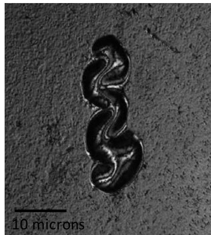
Film E – localised 'telephone cord' buckles
