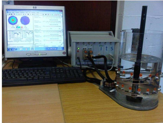
Figure 1.2 ITS, P2000 Electrical Resistance Tomography System at City University London.
