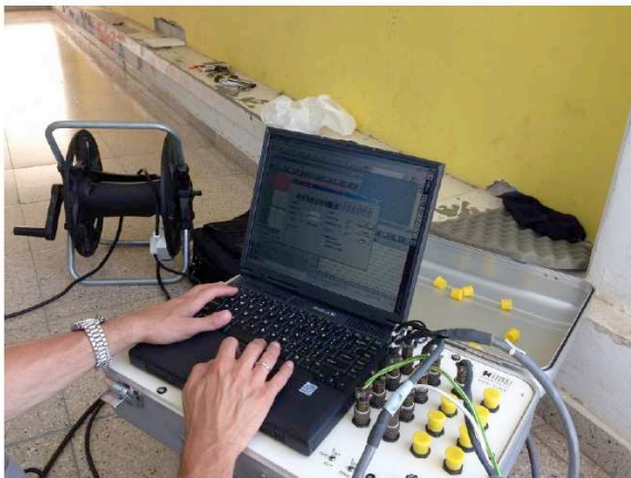
Fig. (27). Wired network recording unit.
