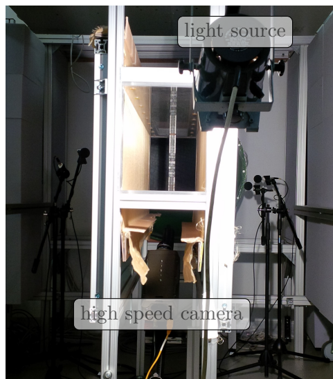
(b) Downstream view, showing the setup used for the measurement of the flap motion
