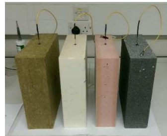
Figure 4. Experimental setting of four types of insulation materials (FLTR: Mineral wool, PIR, Phenolic, BPS), each inserted by a humidity sensor.
