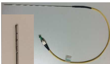
Figure 3. The humidity sensor packaged with perforated stainless steel tube (20cm length, 1mm outer diameter and 0.2mm wall thickness).
