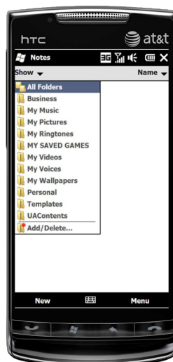
Figure 1: HTC PURE Windows mobile 6.5 displays a WIMP-GUI like menu within a small screen (source: Lina Pio - twitter @linapio - London, March 2012). The Berne Convention allows the non-profitable use of software print screens.
