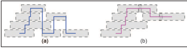
Figure 9. Two layout algorithms. Each rectangle is the bounding box of an event with its label (a) Completeness algorithm: \theta = 1, \gamma = 5/3 . (b) Traceability algorithm ( t_{\min} = 0.5, r_{\max} = 1 ): \theta = 6/7, \gamma = 2/3 .
