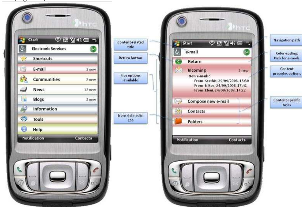
Fig. 1. Mockup of the main menu and the e-mail services for the mobile device. The identified generic guidelines/requirements have been appended to the mockup
