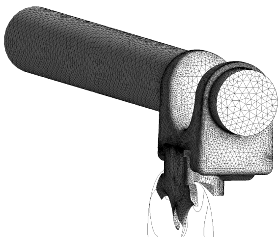
Figure 5. Solver-1 Tetrahedral Mesh
