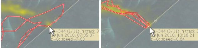
Figure 9: Moving the mouse pointer over the density plot provides a tooltip whenever over an original data point (same dyke as in Fig. 7). If multiple data points are at that location, left/right clicking with cycle forward/backwards through these and any associated journey if one exists.
