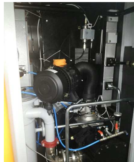
Figure 11 Water injected compressor prototype under testing
