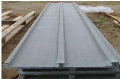
Fig.15. An extruded SHCC panel
