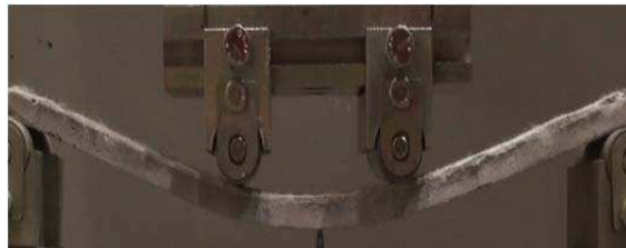
Fig.3. High flexural deformation of SHCC
