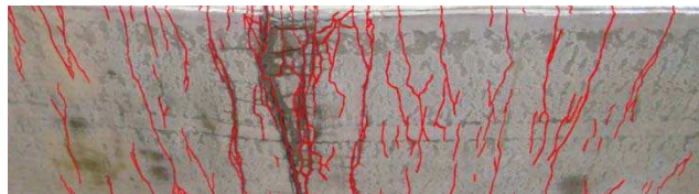
Fig.17. Multiple micro-cracks and failure pattern of specimen EXT1-P1
