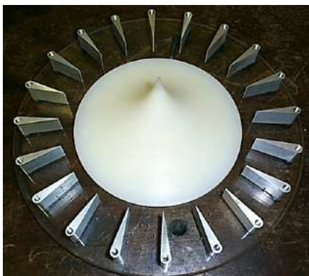
Figure 1: The assembly of the rotating orifices
