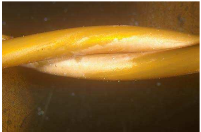
Figure 3. Damaged area: Nanocomposite Enamel, 65% RH, 9000 V
