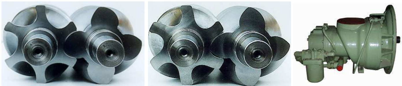
Fig. 2 Rotor retrofit in oil-flooded screw compressors, old rotors left, new rotors, right, Stosic et al, 2000
