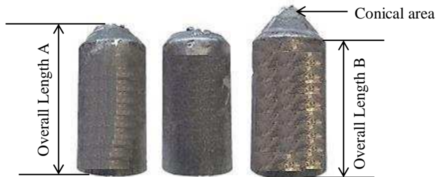
Figure 2: Several example of the formed billets which occurred after the injection test. The overall length of the billets was measured from bottom to maximum height of the feedstock billets.
