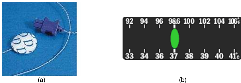
Figure 5.8: (a) A thermocouple skin temperature sensor (Image credit: http://www.arizant.co.uk/ ); (b) A liquid crystal temperature sensor (Image credit: http://www.novamed-usa.com )
