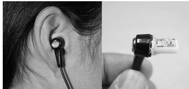
Fig. 4. Photograph of the ear canal PPG/ SpO_2 probe placed inside the right ear of a volunteer.
