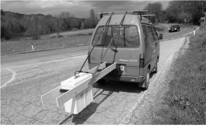
Figure 2. The GPR survey van.
