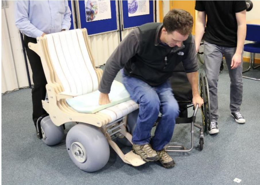
Figure 2: Testing the sand chair prototype for ease of transfer to a wheelchair
