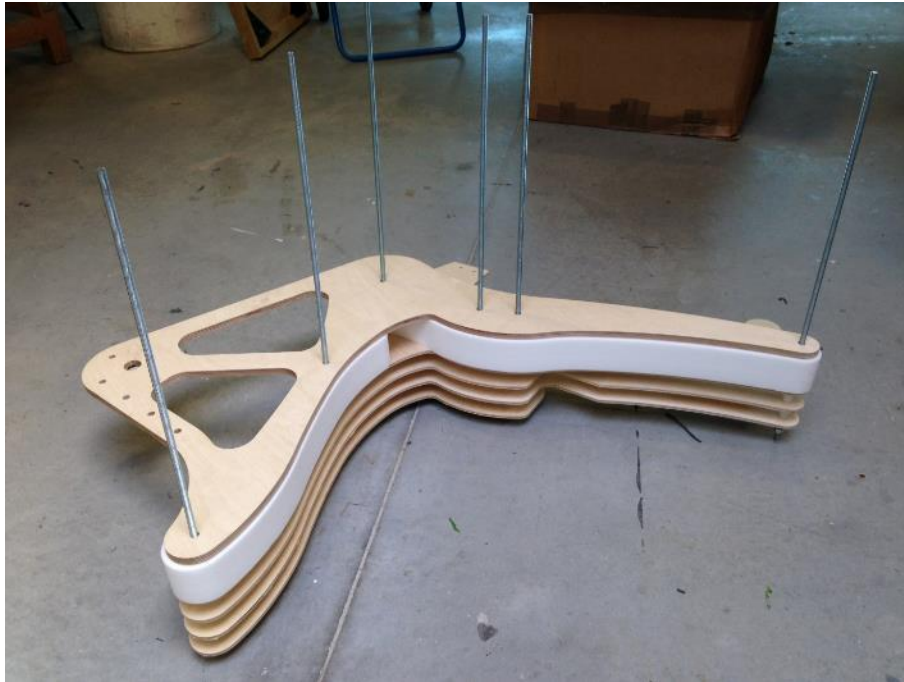
Figure 5: Plywood and EVA foam prototype partially assembled
