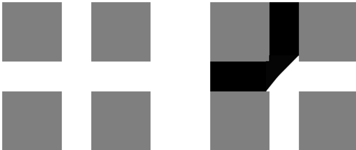
Figure 3. (a) Schematic depiction of an empty, ‘+’ shaped intersection in a model pore bond network (shown in white), and (b) following partial retraction and subsequent entrapment of mercury (shown in black).
