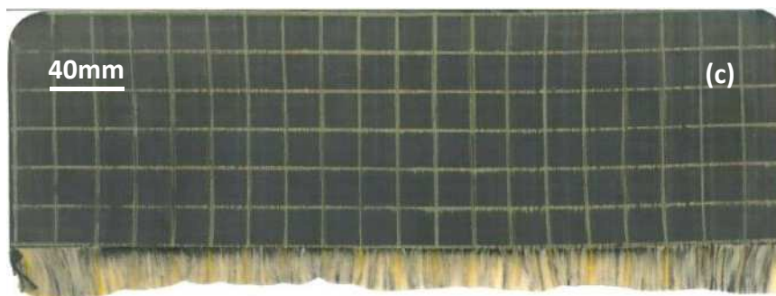
Figure 4: (a) Optical micrograph of a polished section from UD3/0°/SMC2/60% showing a split in the top three plies of UD. (b) Optical micrograph showing the distribution of the yellow paint marker used to define the grid for the photogrammetry study. (c) Surface scan of UD3/0°/60% showing migration of resin.
